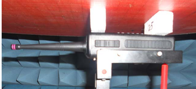
Figure 7.2: DUT position during the tests in Front of Face condition
