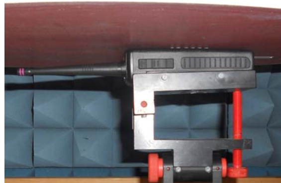
Figure 7.3: DUT positions during On Body and Hand Use conditions. Left: DUT's back towards the phantom, right: DUT's front towards the phantom
