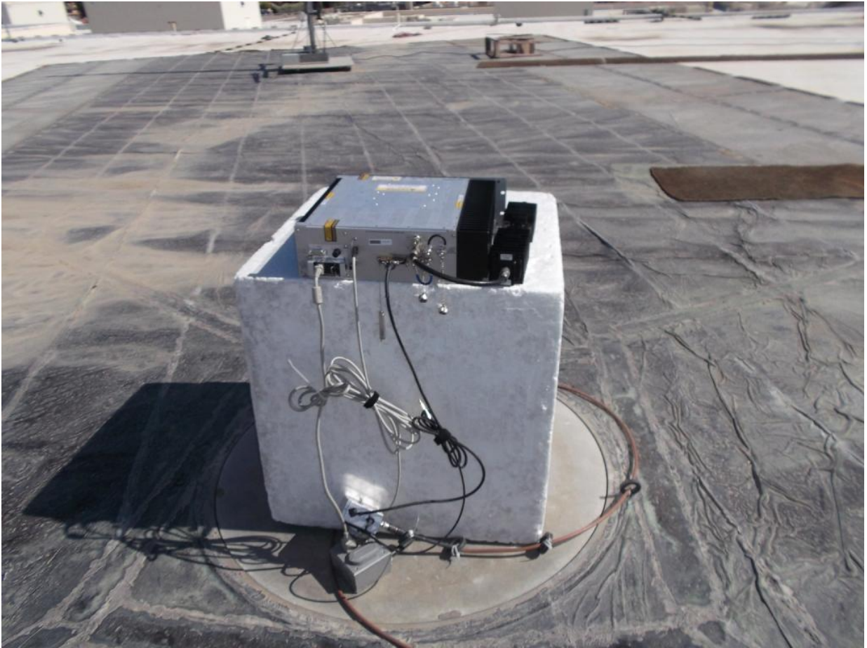
Figure 7.0-4 Radiated Emissions Test Setup (OATS)
