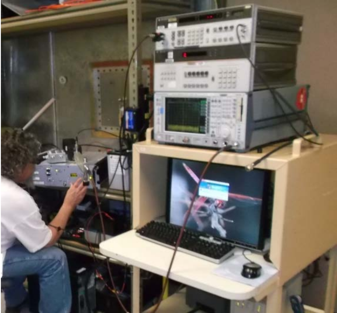
Figure 7.0-6 Front-End Conducted Emissions Test Setup
