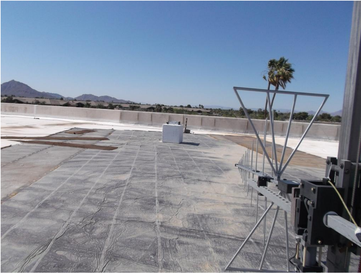
Figure 7.0-5 Radiated Emissions Test Setup (OATS)
