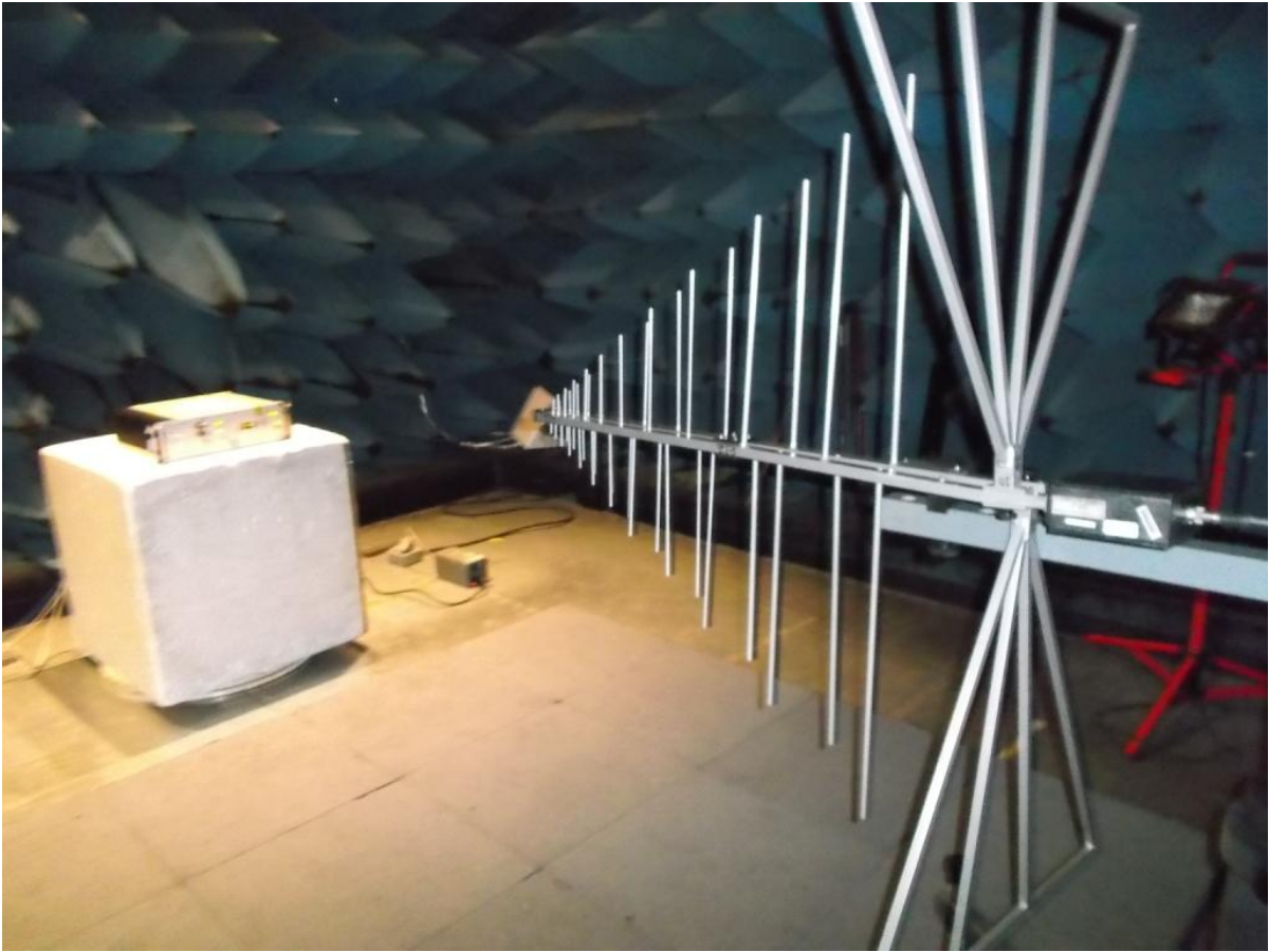
Figure 7.0-3 Radiated Emissions Test Setup (Pre-Scans/Anechoic Chamber)
