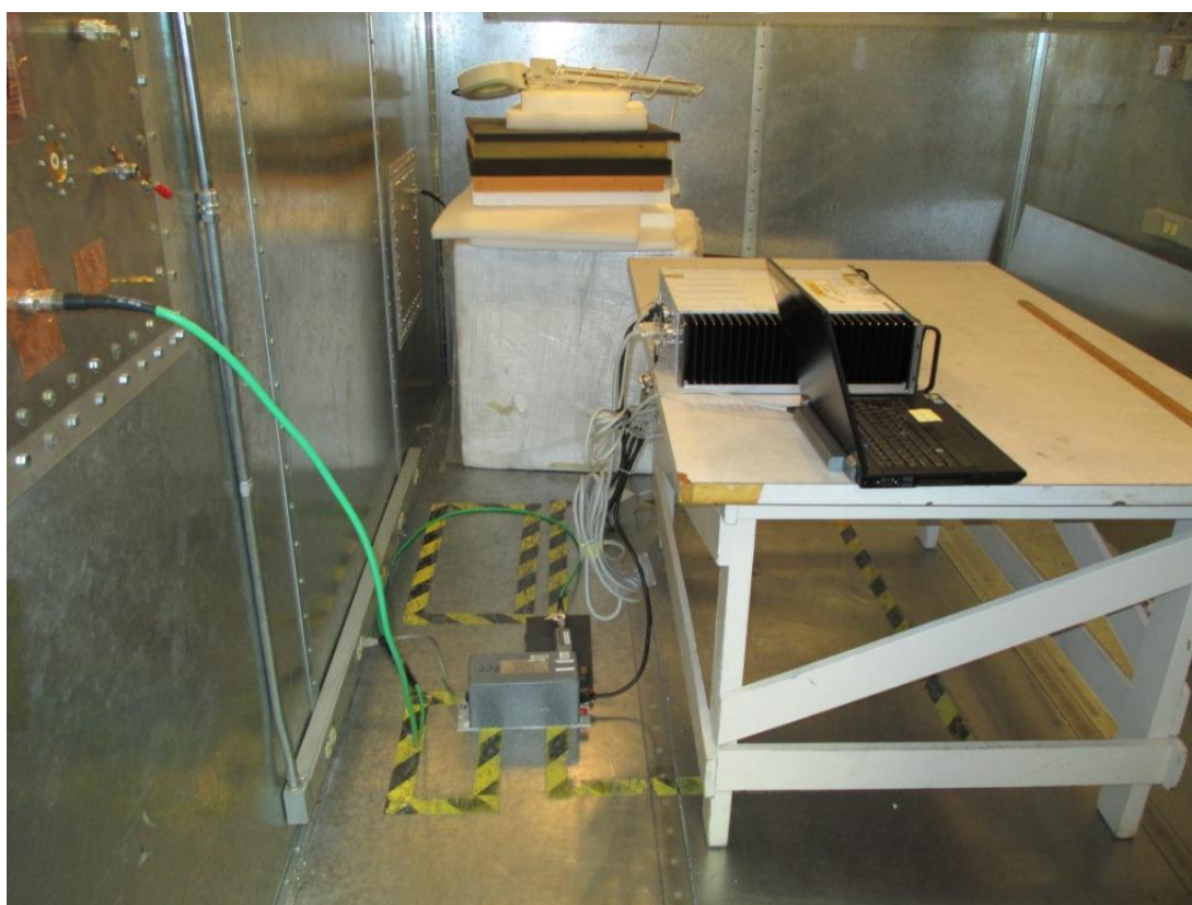
Figure 7.0-1 Conducted Emissions Test Setup
