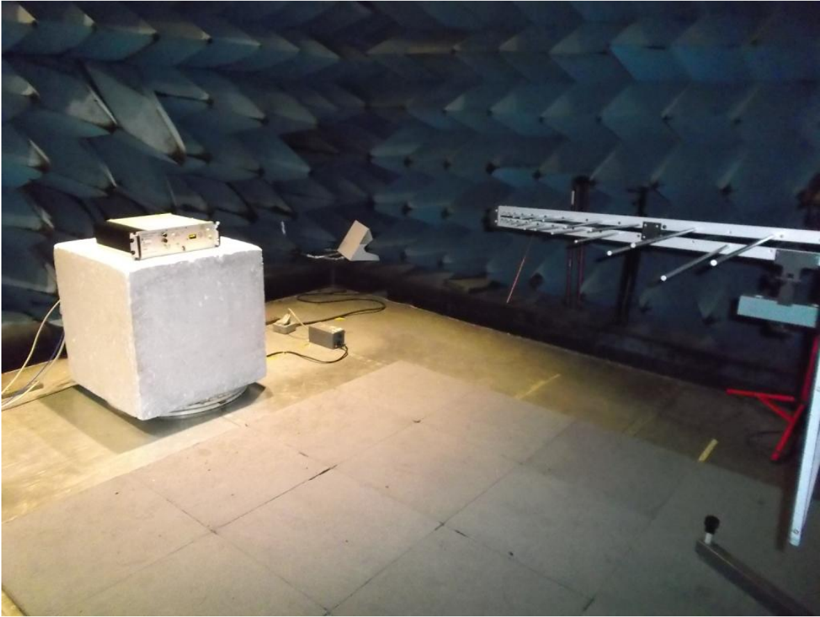
Figure 7.0-2 Radiated Emissions Test Setup (Pre-Scans/Anechoic Chamber)
