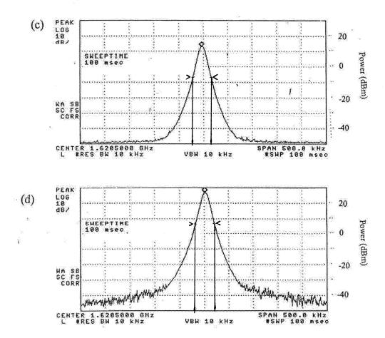
Figure A3. TX amplifier responses (continued). (c) High level input signal to the TX amplifier, (d) output from amplifier. The gain of the amplifier is 14.0 dB, span of spectra is 500kHz and video bandwidth of EMC meter 10kHz. Output of amplifier is 27dBm as required.
