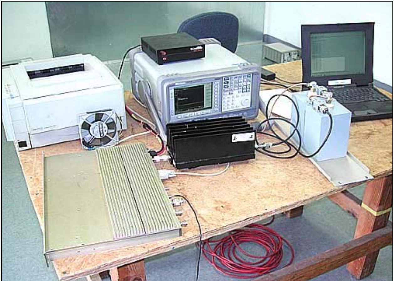
PHOTOGRAPH SHOWING ADJACENT CHANNEL POWER
