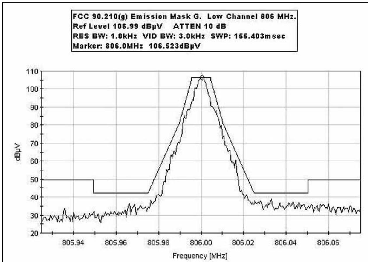
**FCC 90.210(g) EMISSIONS MASK LOW CHANNEL (806 MHz) 1 M Span**
