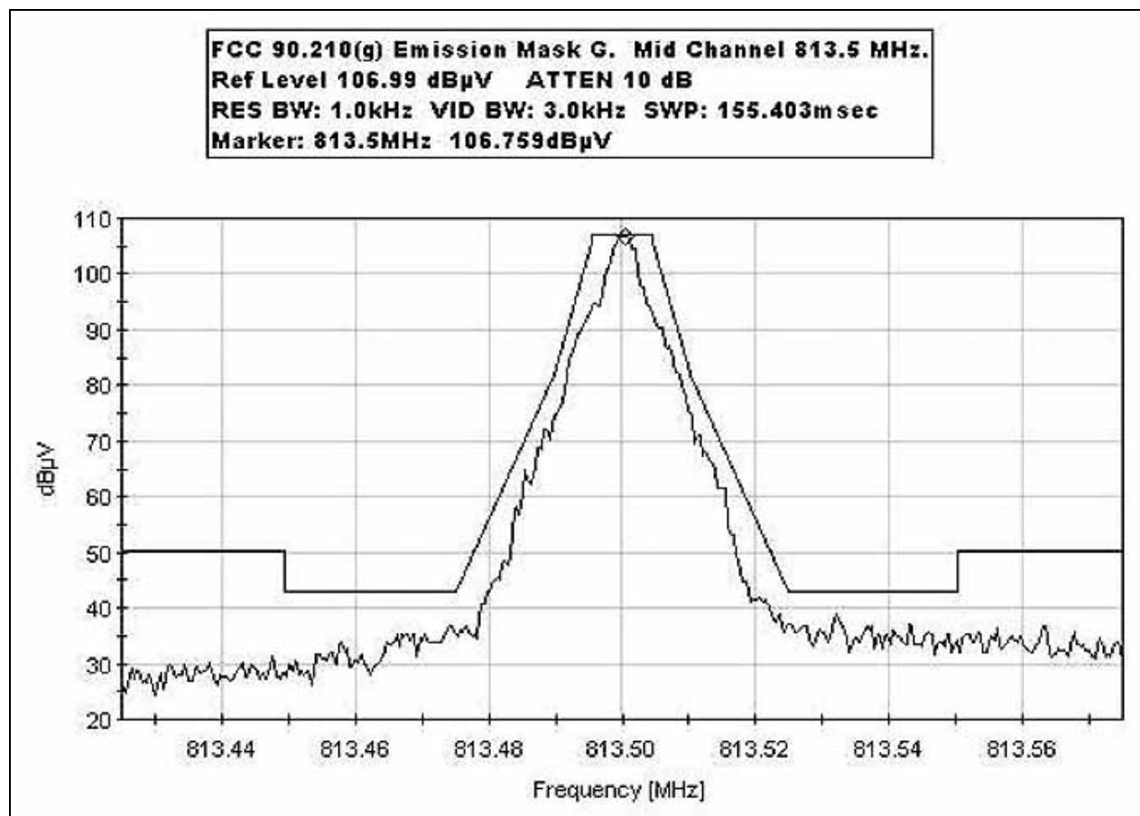
**FCC 90.210(g) EMISSIONS MASK MID CHANNEL (813.5 MHz) 1 M SPAN**
