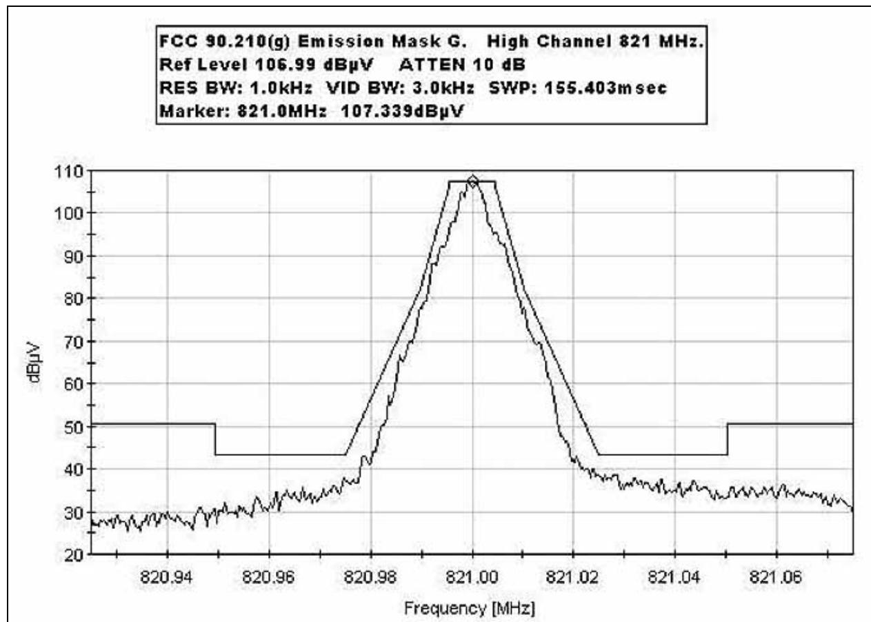
**FCC 90.210(g) EMISSIONS MASK HIGH CHANNEL (821 MHz) 1 M Span**
