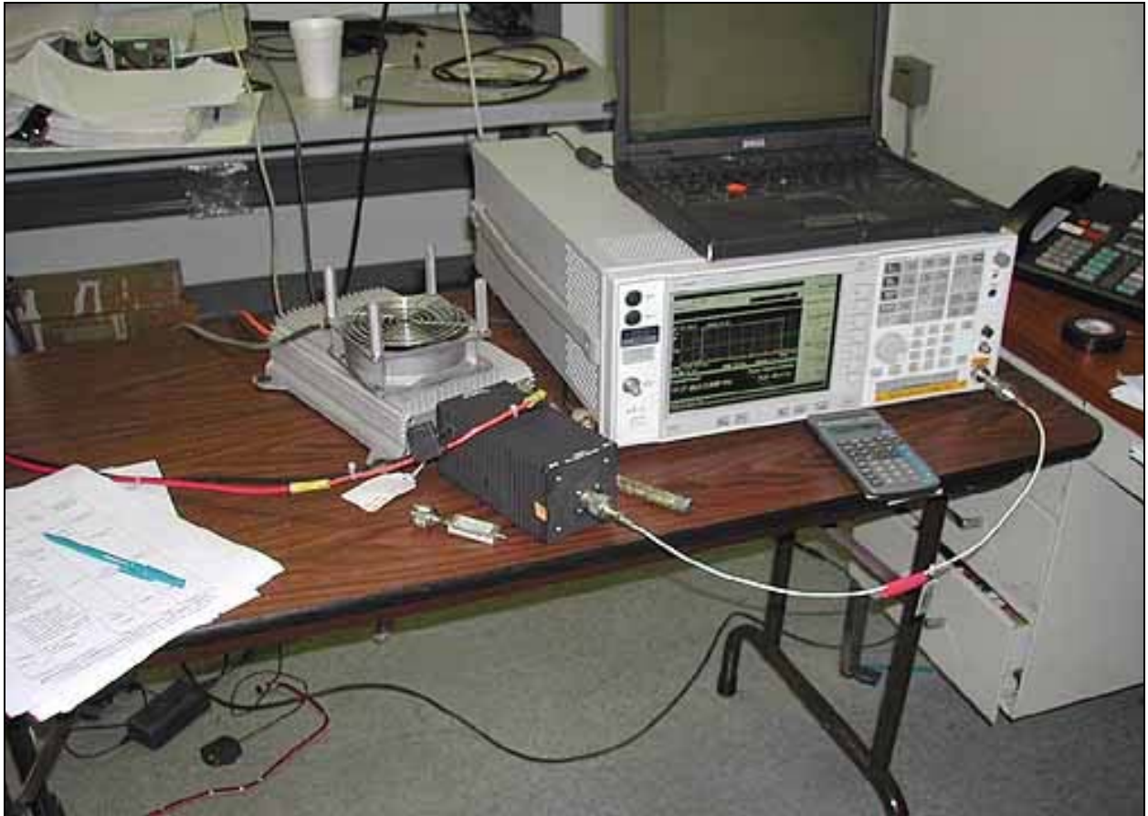
PHOTOGRAPH SHOWING DIRECT CONNECT TEST SETUP
