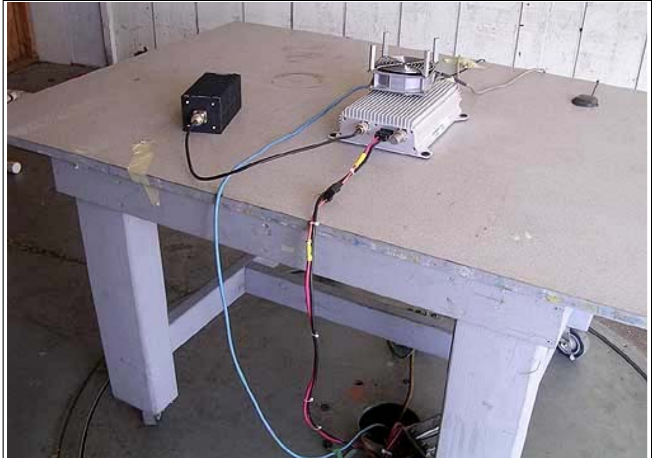
Radiated Emissions - Front View
