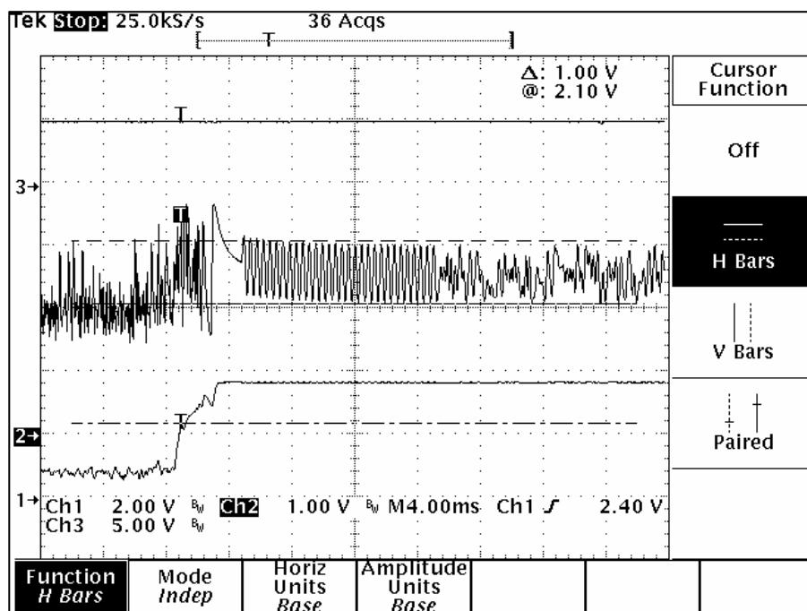
As can be seen from this plot, the base station's transmit carrier has ramped up to full power (Channel 1) in just a few milliseconds. The recovered modulation (Channel 2) is stable by this time. There follows a few milliseconds of quiet time followed by 12 milliseconds of symbol sync time.
