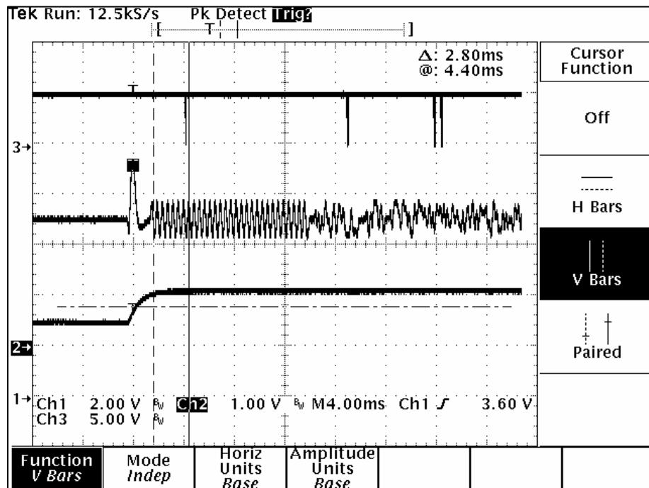
The recovered modulation should be centered at approximately 2.5 VDC and should have the amplitude of approximately 800 mV peak-to-peak as indicated in the plot above.
