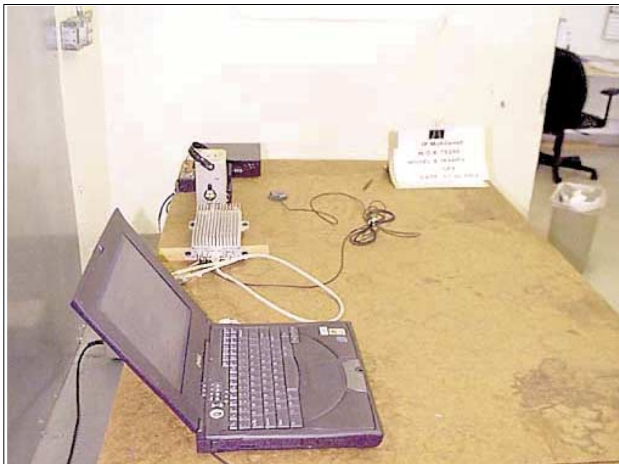
Mains Conducted Emissions - Back View – UTP
