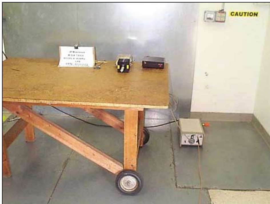
Mains Conducted Emissions - Front View - RS232
