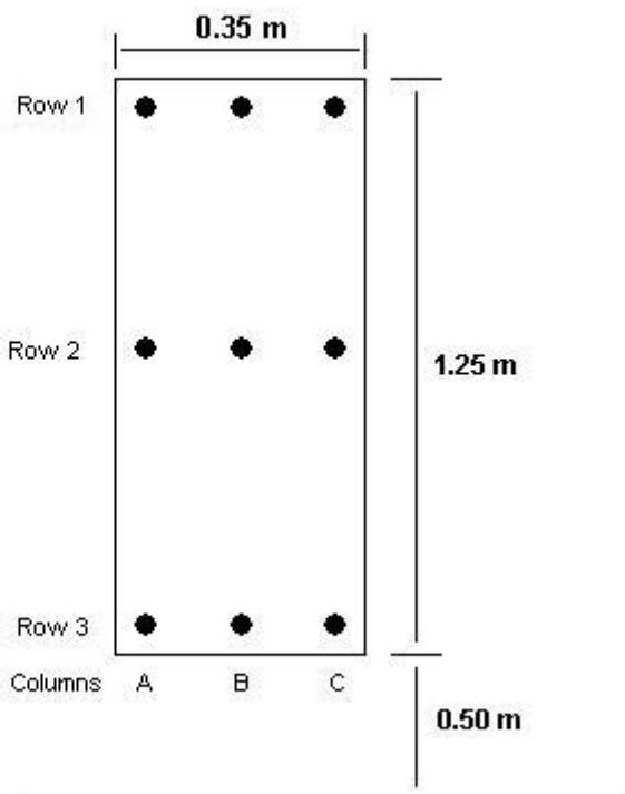
The following diagram is an example of the setup used for most tests, excluding magnetically mounted vehicle antennas.
