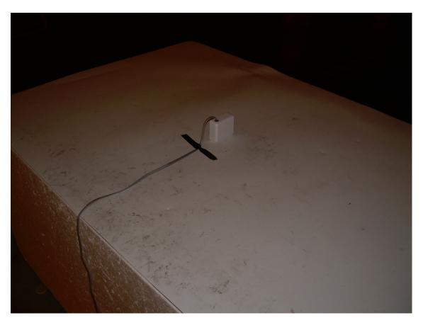
Back View Radiated Disturbance Worst Case Configuration On-Edge Placement
