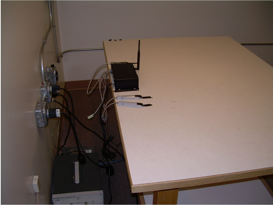
Back View Conducted Disturbance Worst Case Configuration
