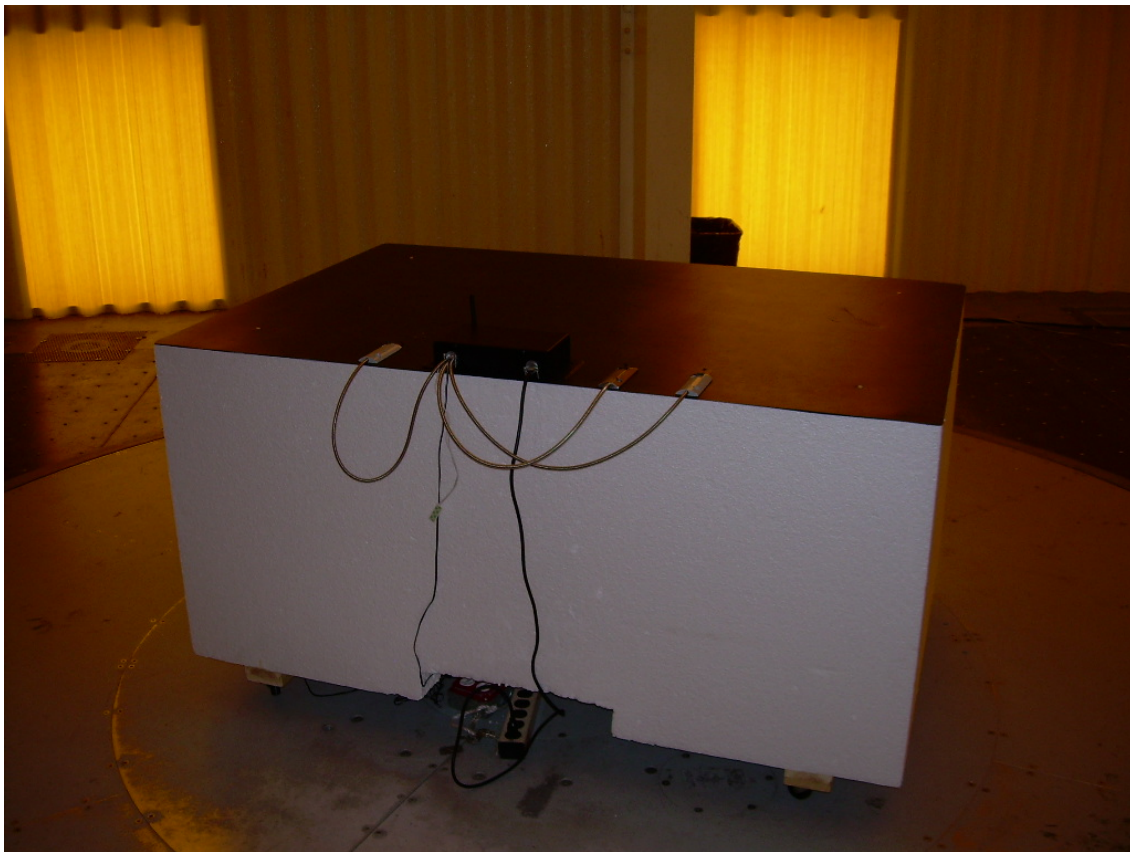
Back View Radiated Emissions in Restricted Bands Configuration
