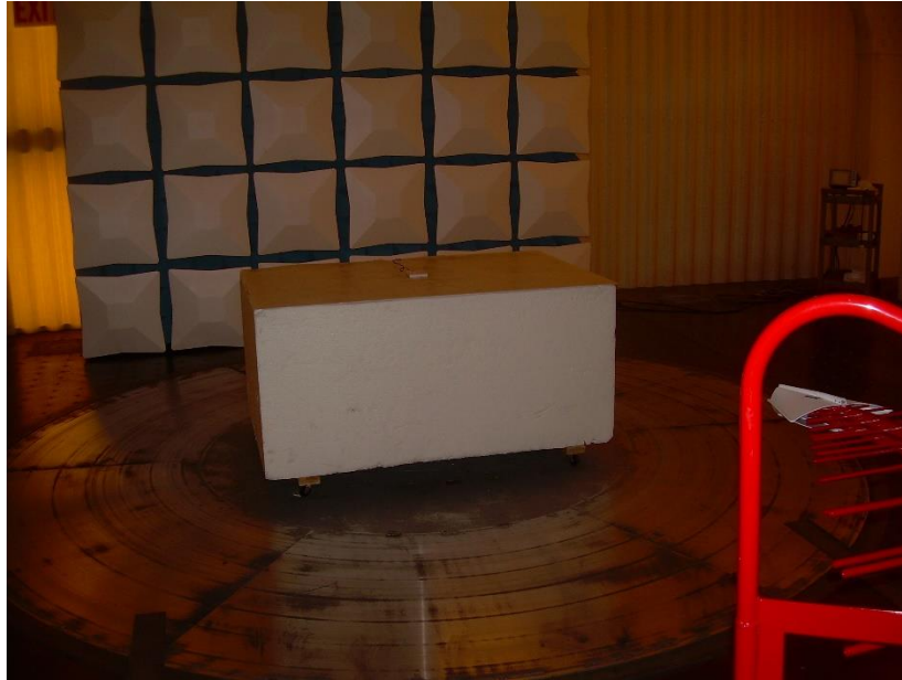
Photograph 1: Front View Radiated Emissions Worst-Case Configuration – 30 to 1000 Mhz
