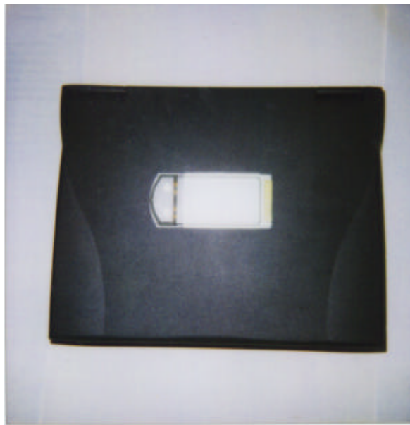
Fig. 2. A picture of the Model CAWCB500 CardBus card placed on the laptop computer.
