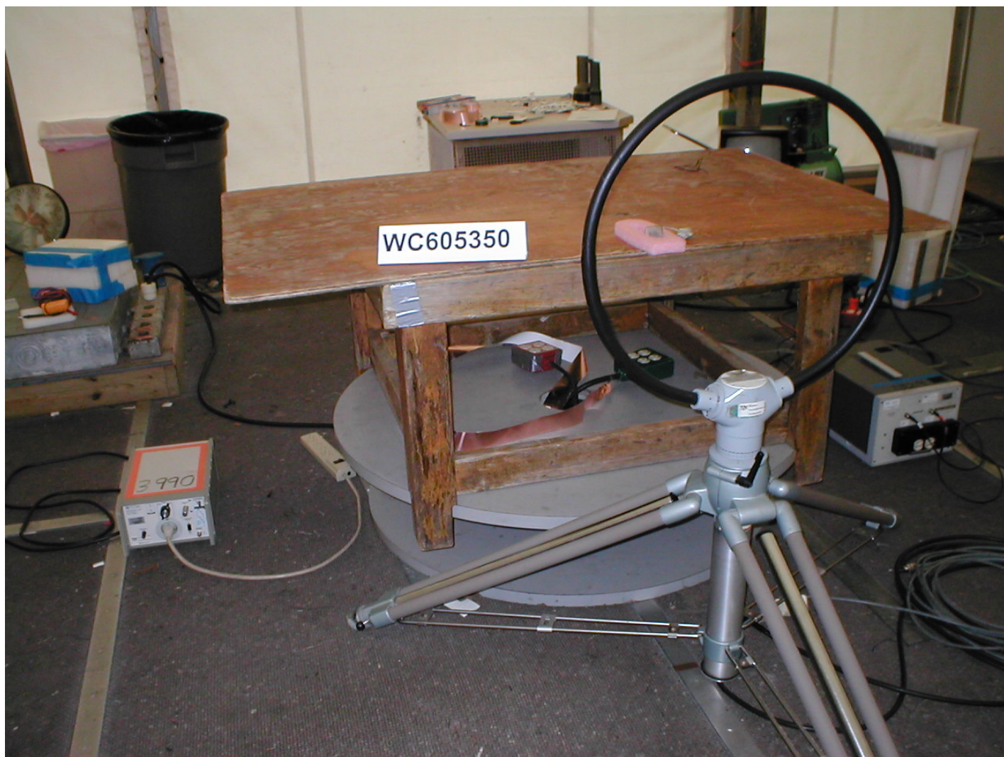
Test-setup photo(s): General Field Strength Limits 0.009 – 30 MHz
