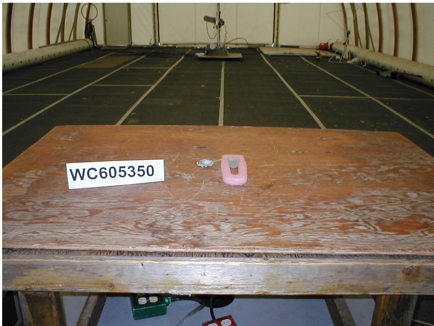
Test-setup photo(s): Radiated Emissions 30 - 1000 MHz
