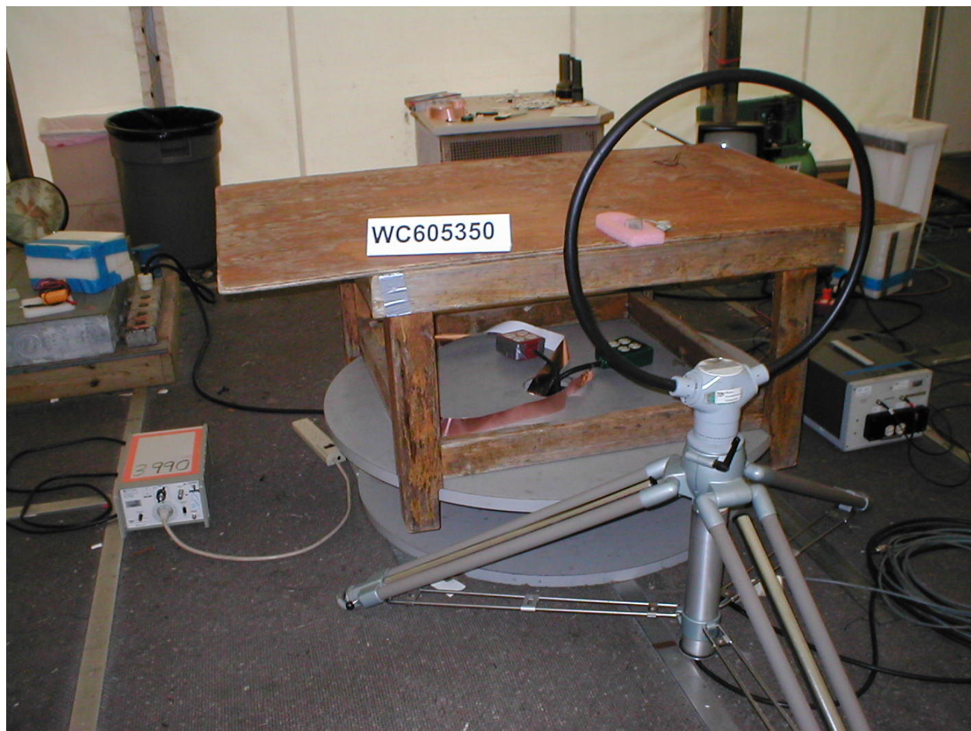
Test-setup photo(s): General Field Strength Limits 0.009 – 30 MHz
