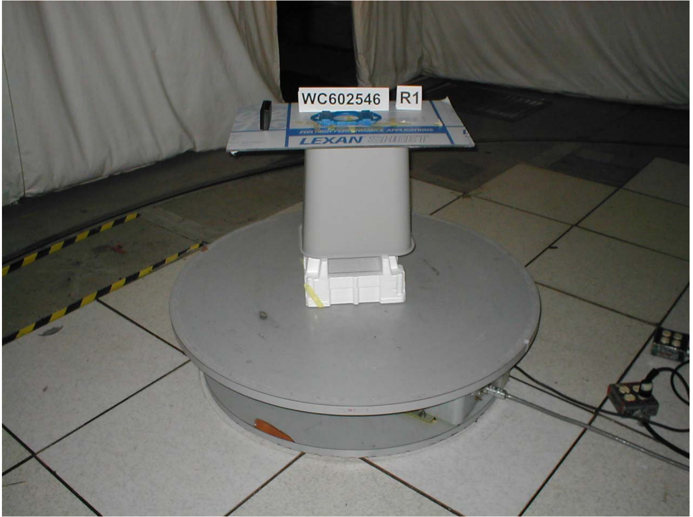
Test setup photo, radiated emissions Repeater RPT-910-3
