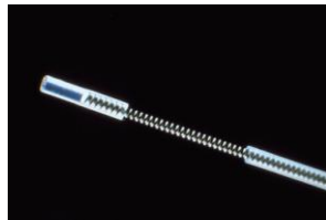
Photo of leads with tip covers placed appropriately
