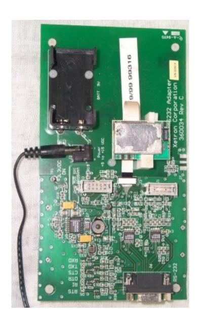
Photo 3. Bottom View of Interface Board Used for Testing
