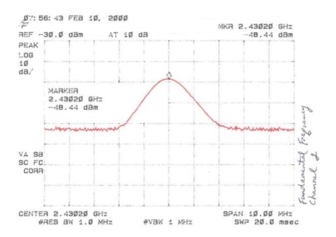
Figure 3c. Field Strength of Fundamental Emissions 15.249(a) (High)
