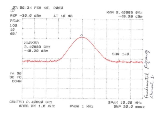
Figure 3b. Field Strength of Fundamental Emissions 15.249(a) (Mid)
