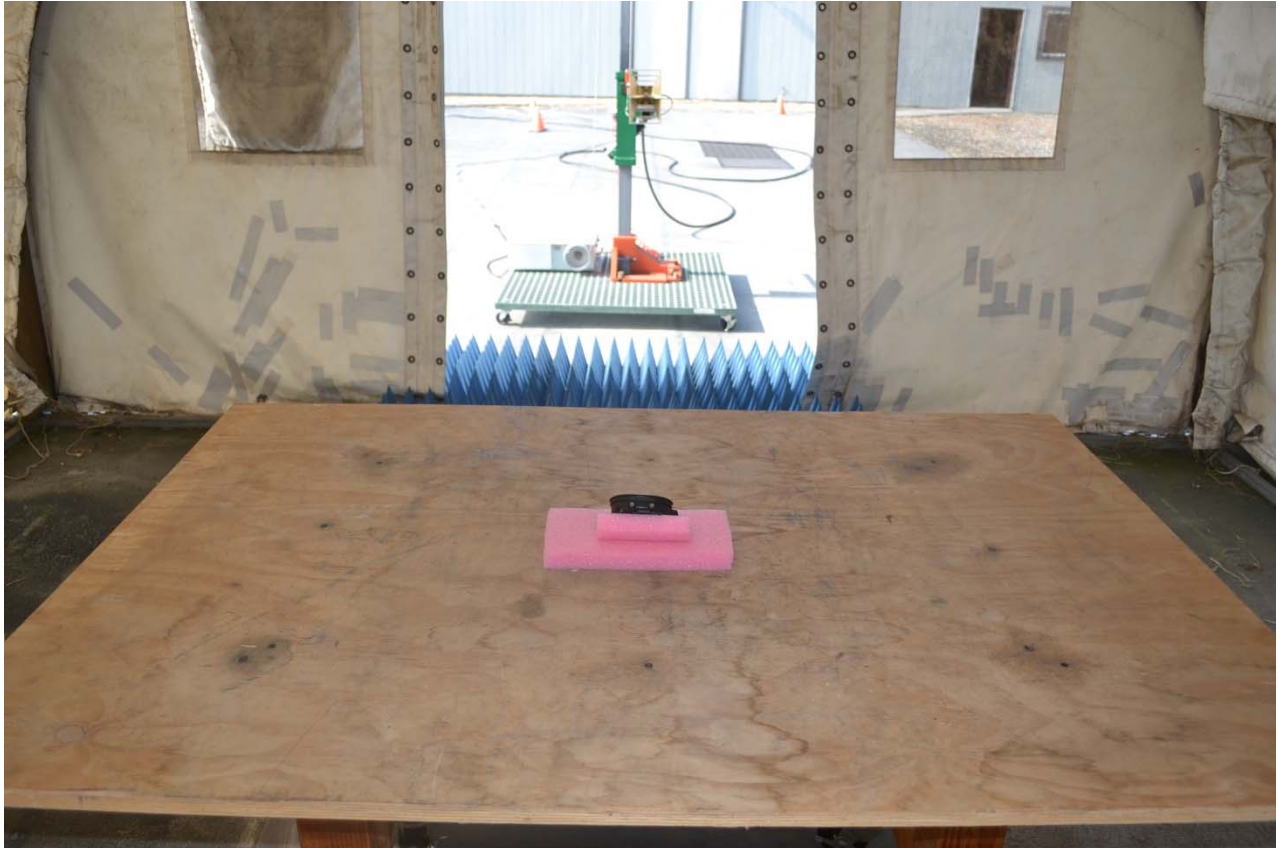
Radiated Emissions Setup (>1 GHz) Model: i550 | NS911279
