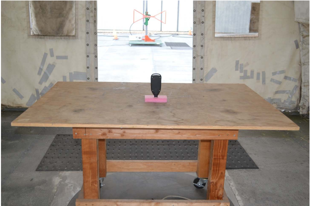
Radiated Emissions (30 – 1000 MHz) Setup: Model: ProplusX | 604.1029.07
