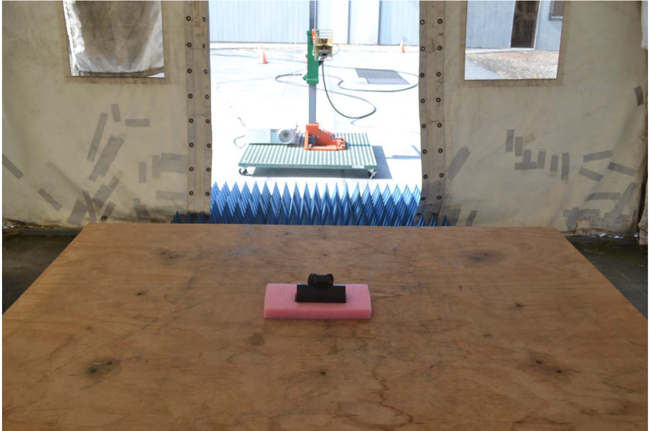
Radiated Emissions Setup (>1 GHz) Model: i750TC | NS118111
