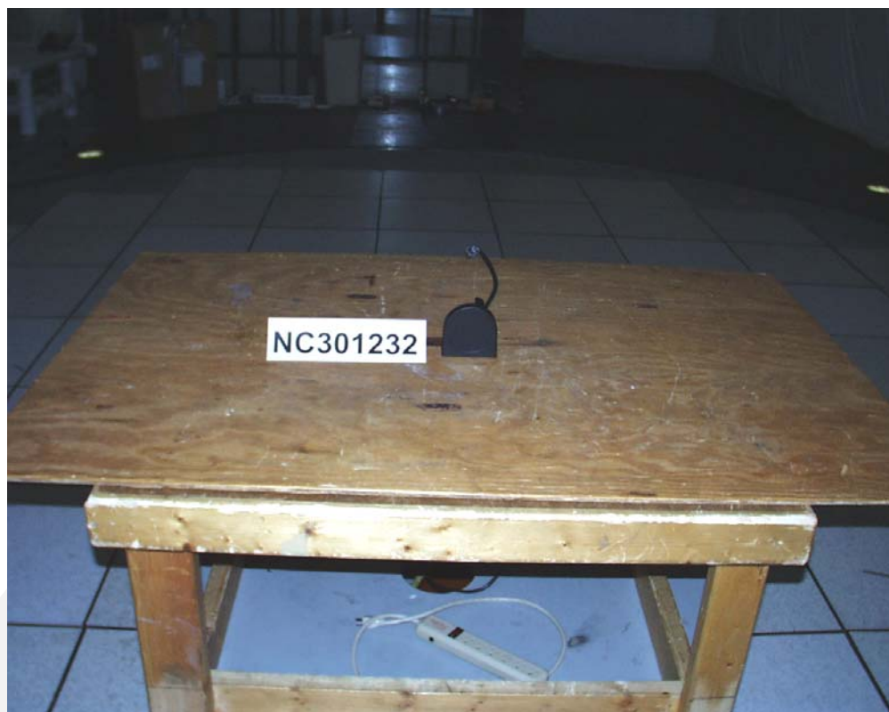
Test-setup photo(s): Radiated emission 30 MHz - 25000 MHz
