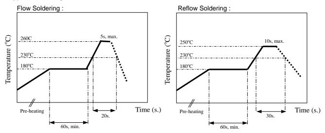
The sample must be pre-heated before soldering .The temperature difference between preheating and soldering must be within 150  $\,^{\circ}$ C.
