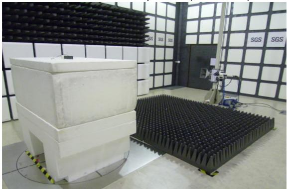
Radiated Emission Set up Photos (Front View)
