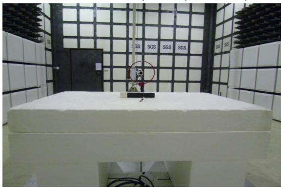
Radiated Emission Set up Photos (Below 1GHz)
