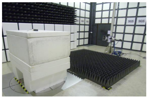
Radiated Emission Set up Photos (Front View)
