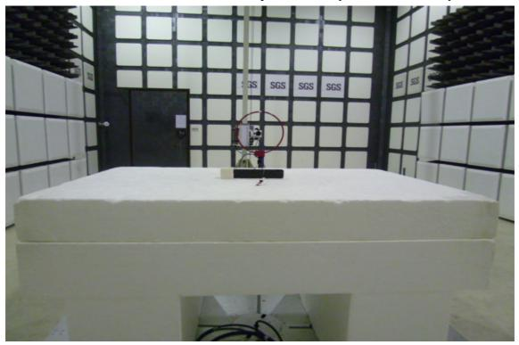
Radiated Emission Set up Photos (Below 1GHz)
