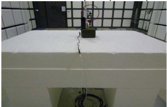
Radiated Emission Set up Photos (Below 1GHz)
