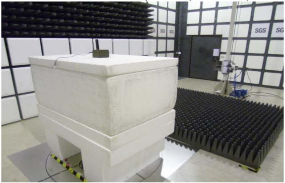
Radiated Emission Set up Photos (Front View)
