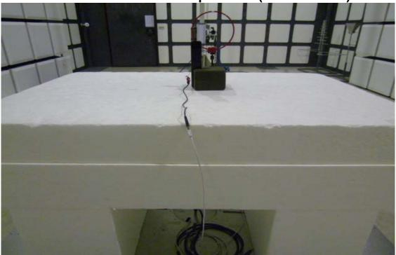
Radiated Emission Set up Photos (Below 1GHz)
