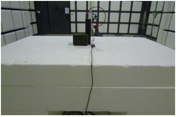
Radiated Emission Set up Photos (Below 1GHz)
