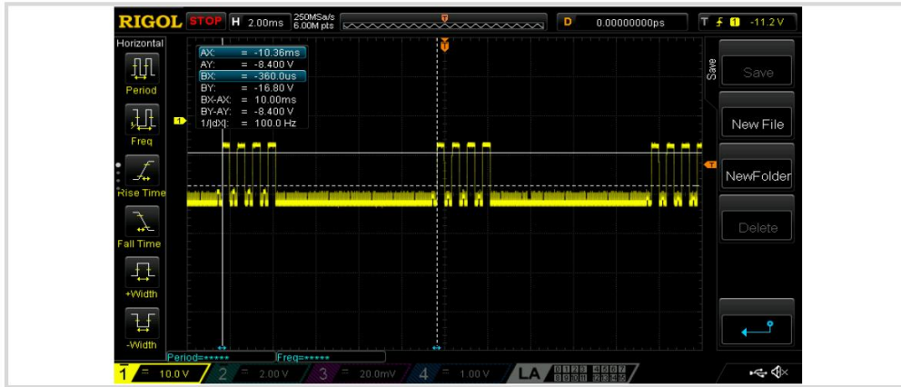
Figure 4 : Oscilloscope Graph of 10 ms Connection Interval
