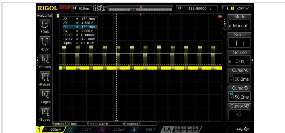
Figure 5 : Oscilloscope Graph 10 ms/div so 120 ms Interval
