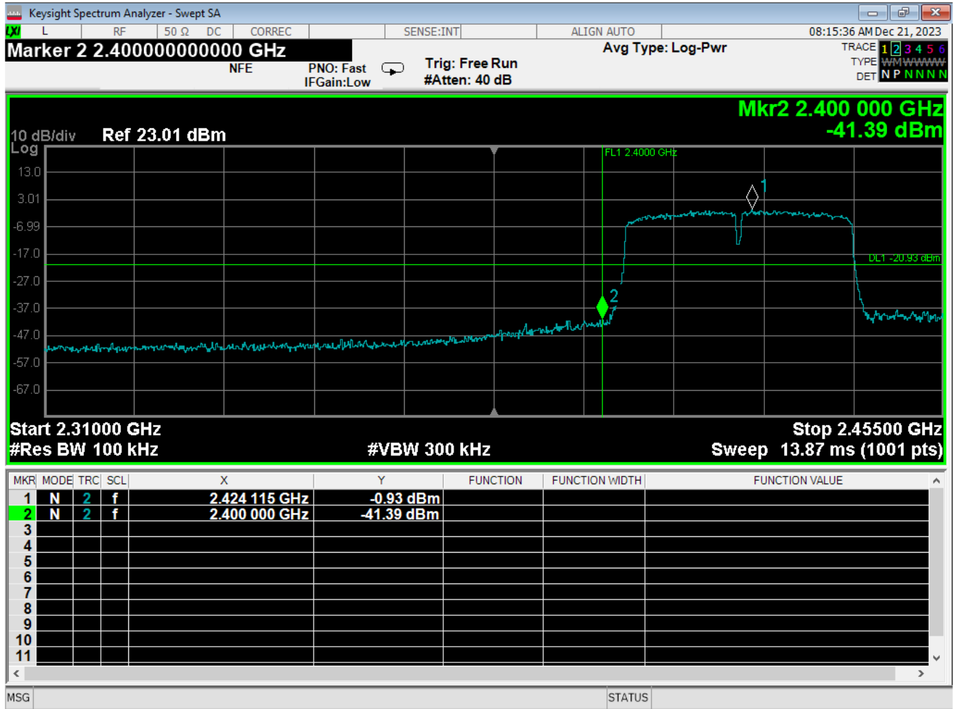
Band Edge – Conducted Measurement at 2400 MHz – 802.11n Mode – 40 MHz
