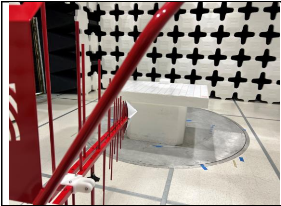
Radiated Emission Test below 1GHz Front View
