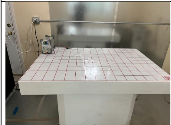
Conducted Emission Front View
