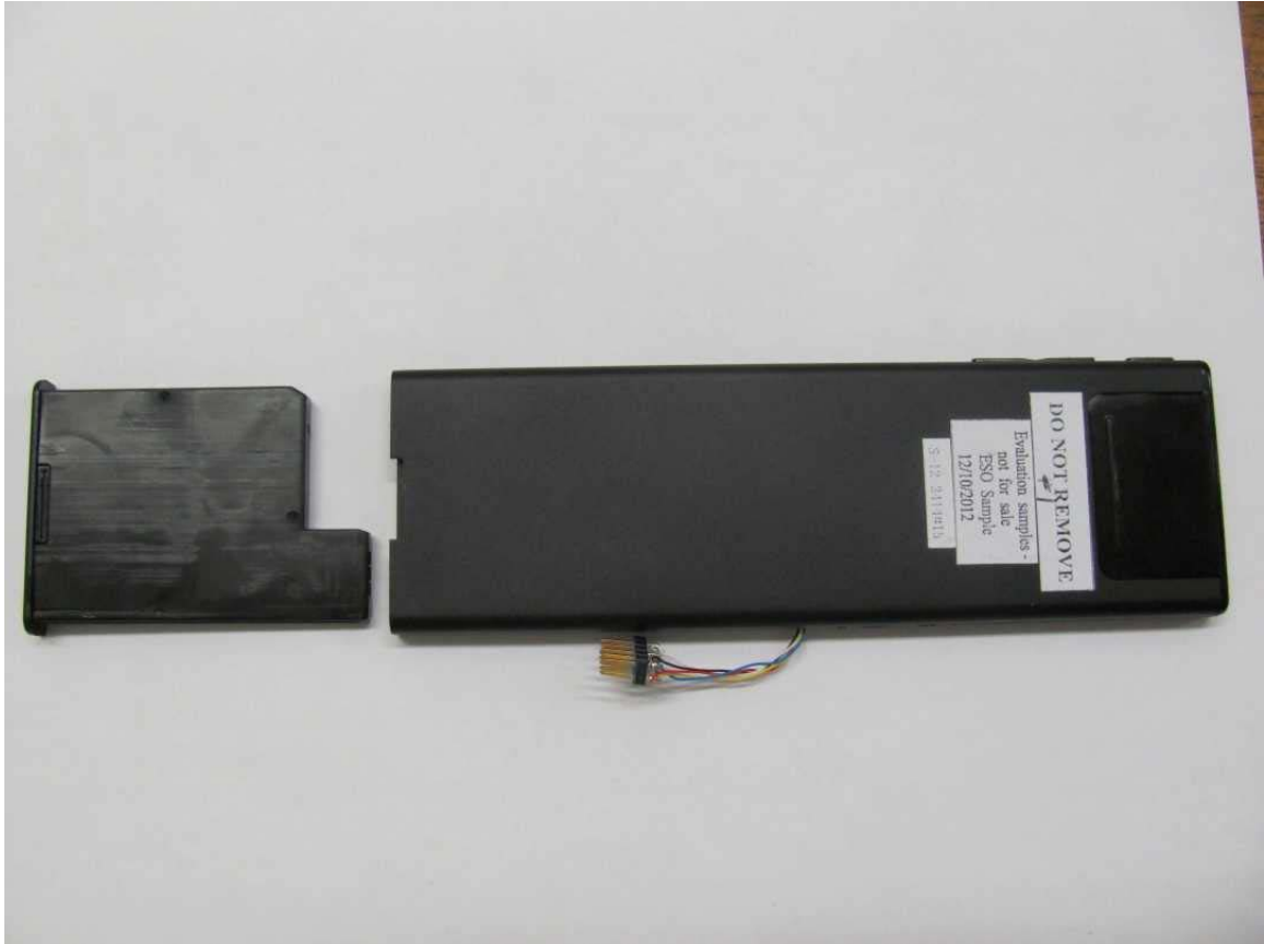
Bottom View with Battery Compartment Exposed
