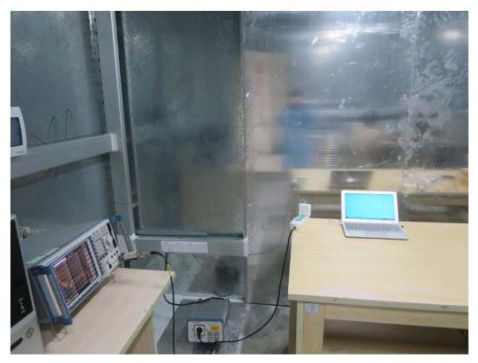
FCC RADIATED EMISSION TEST SETUP
