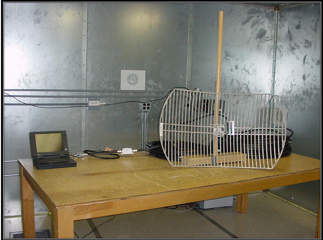
PHOTOGRAPH 4: CONDUCTED EMISSIONS FRONT VIEW WORST CASE CONFIGURATION
