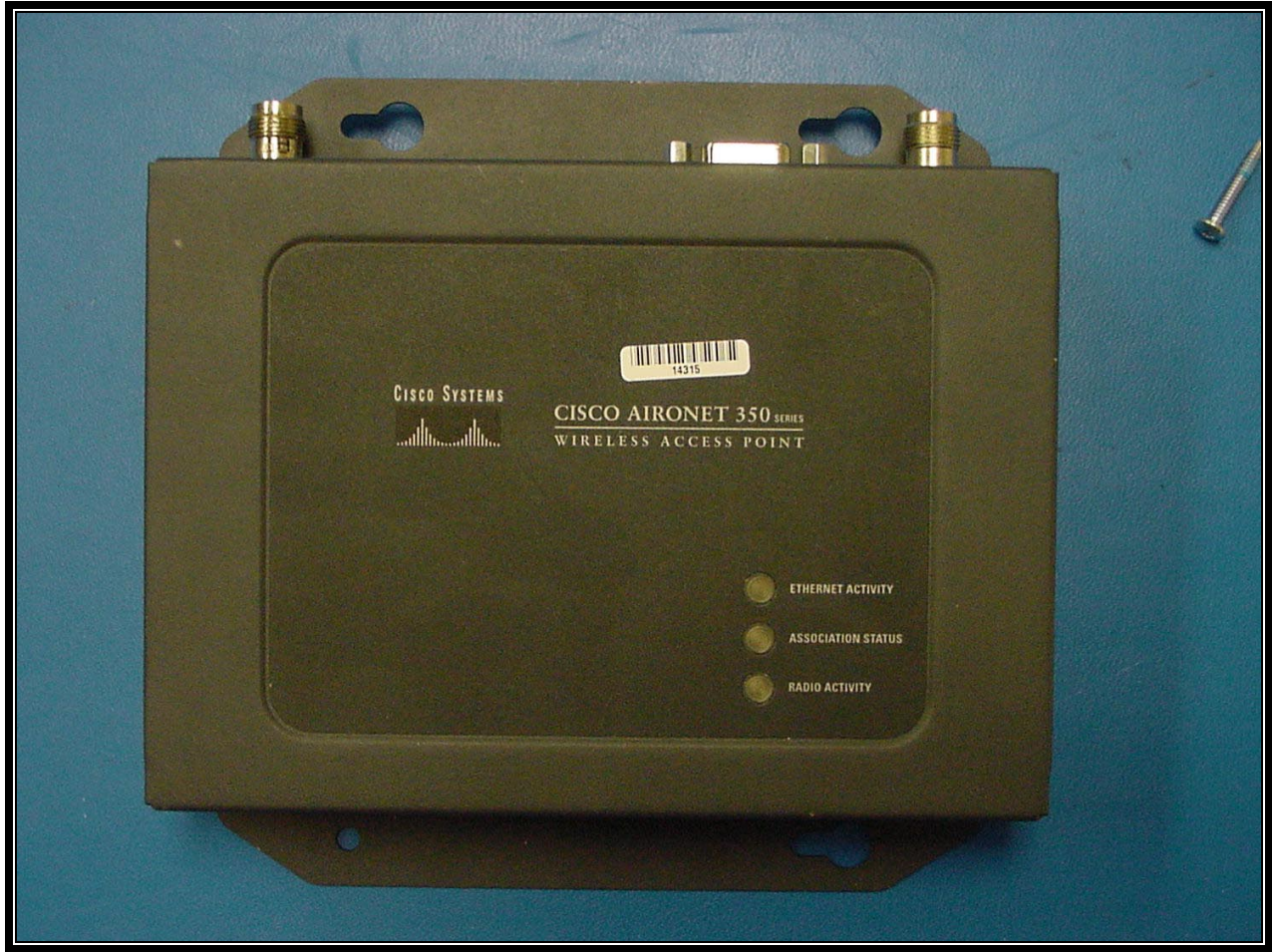
PHOTOGRAPH 17: FRONT VIEW OF ACCESS POINT
