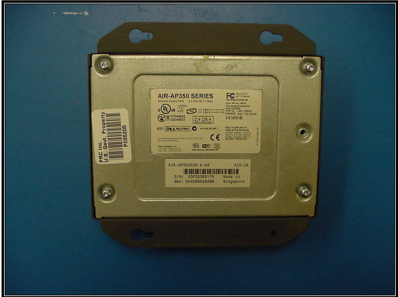
PHOTOGRAPH 18: BACK VIEW OF ACCESS POINT
