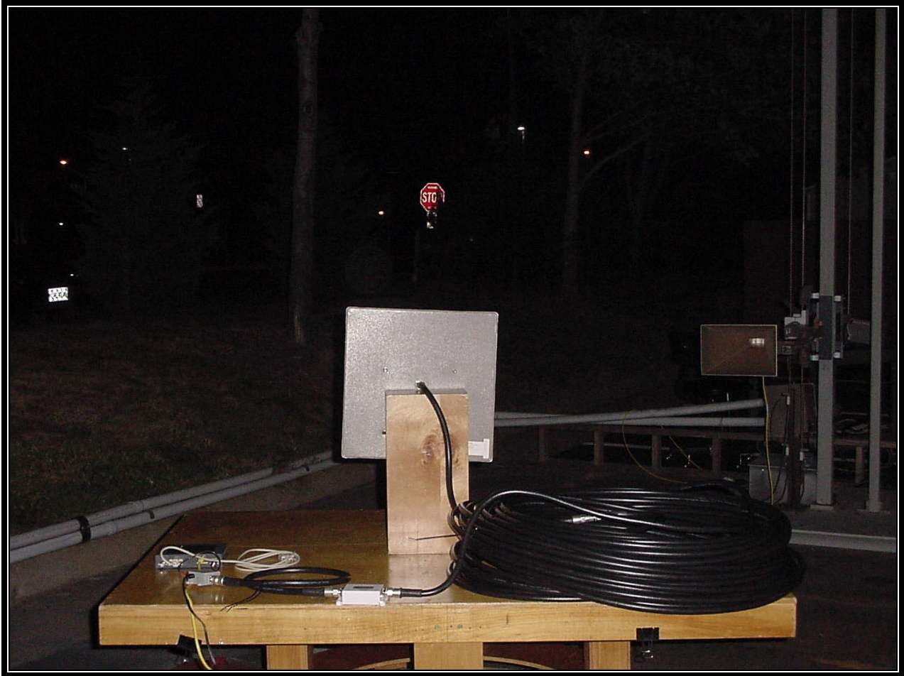
PHOTOGRAPH 10: RADIATED EMISSION FRONT VIEW WORST CASE CONFIGURATION 19 dBi Patch
