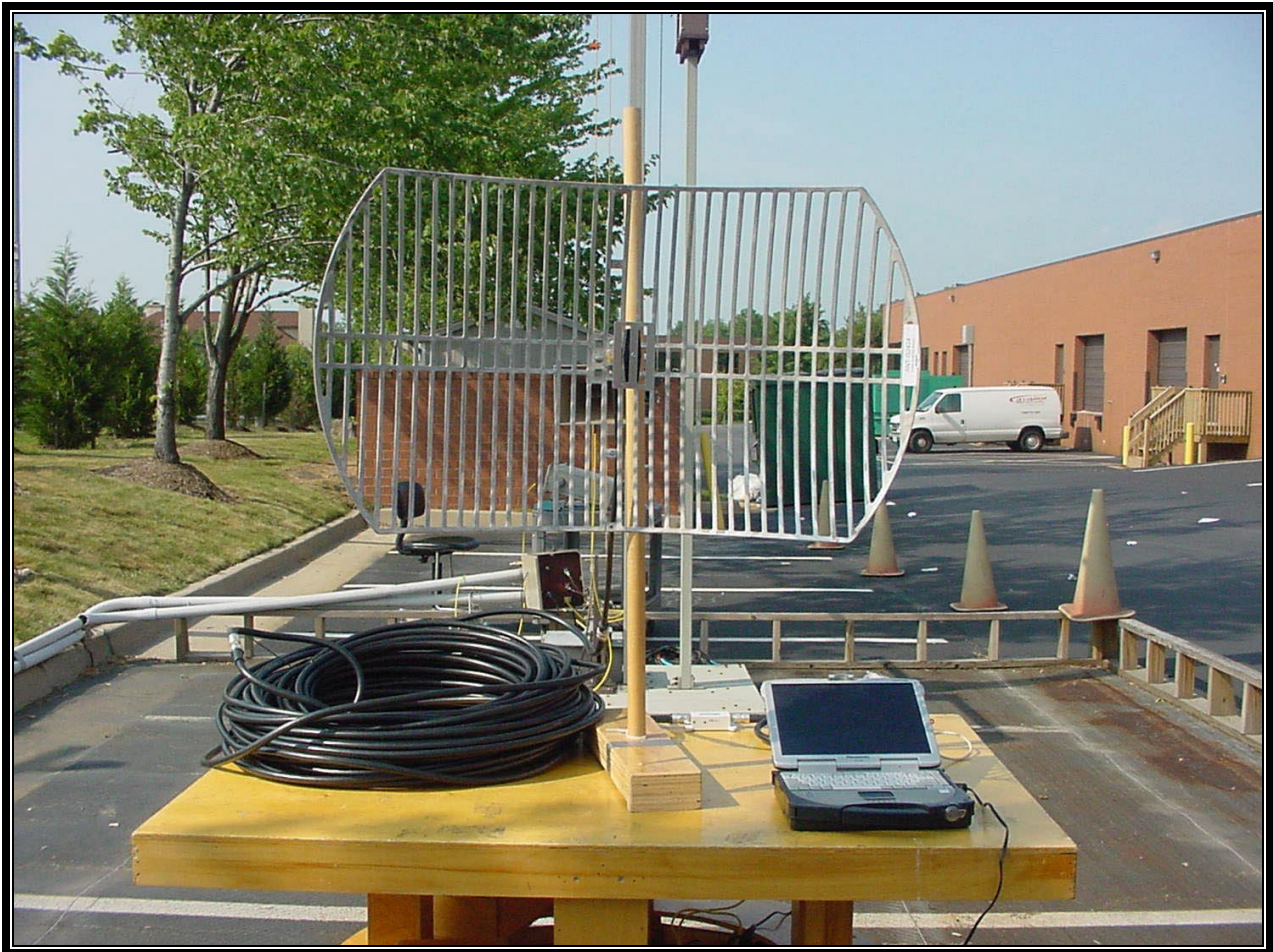
PHOTOGRAPH 14: RADIATED EMISSION FRONT VIEW WORST CASE CONFIGURATION 24 dBi Patch
