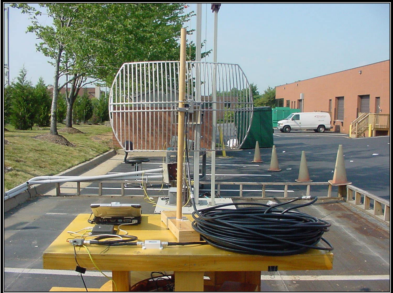
PHOTOGRAPH 15: RADIATED EMISSION REAR VIEW WORST CASE CONFIGURATION 24 dBi Grid
