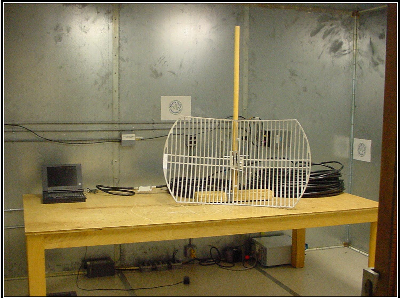
PHOTOGRAPH 18: CONDUCTED EMISSION FRONT VIEW WORST CASE CONFIGURATION 24 dBi RFLCR
