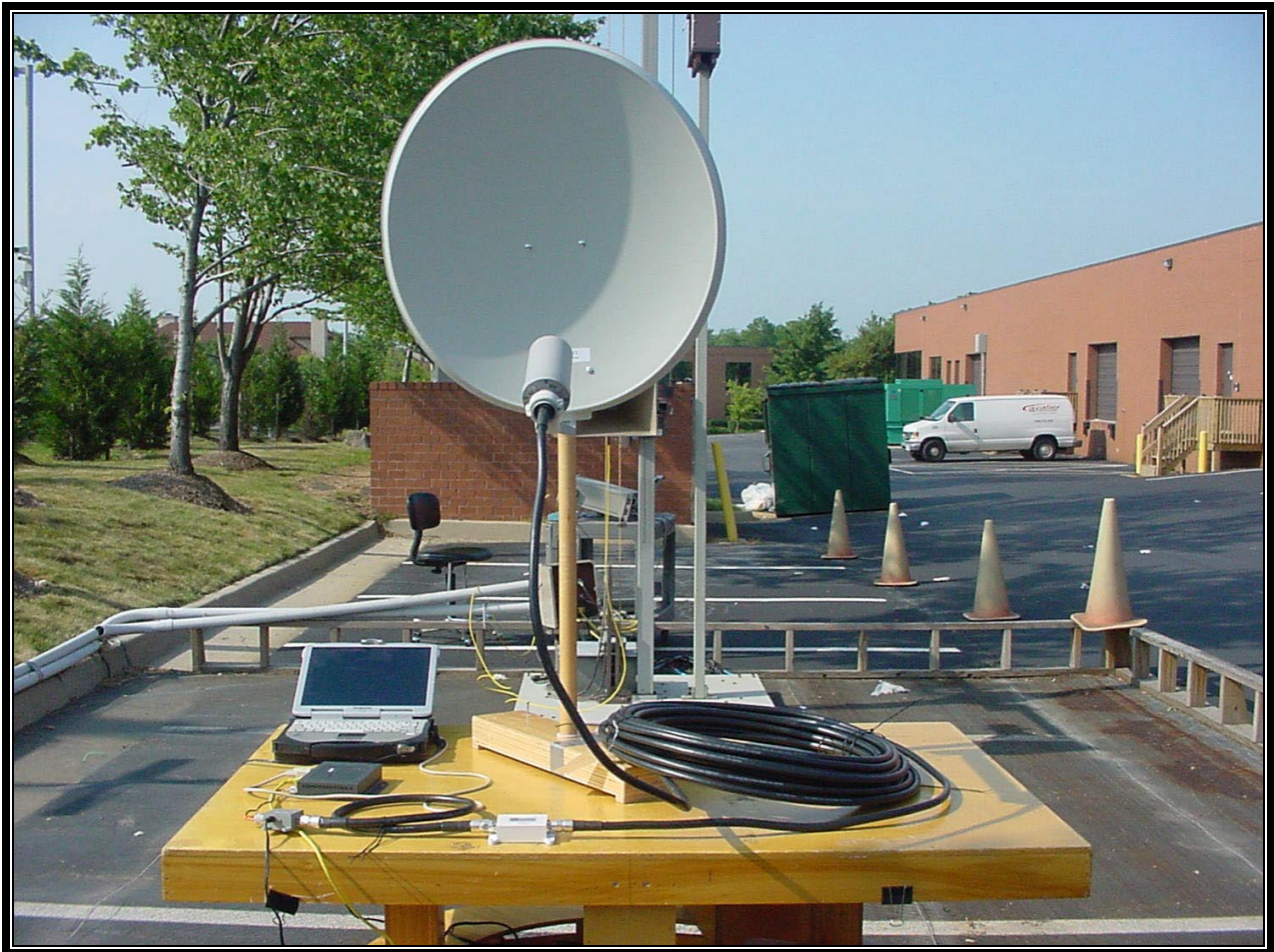
PHOTOGRAPH 16: RADIATED EMISSION FRONT VIEW WORST CASE CONFIGURATION 20.5 dBi Dish
