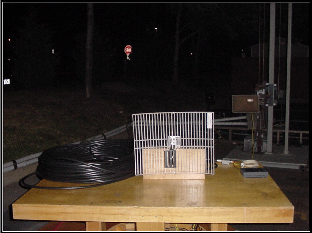
PHOTOGRAPH 12: RADIATED EMISSION FRONT VIEW WORST CASE CONFIGURATION 18 dBi Patch
