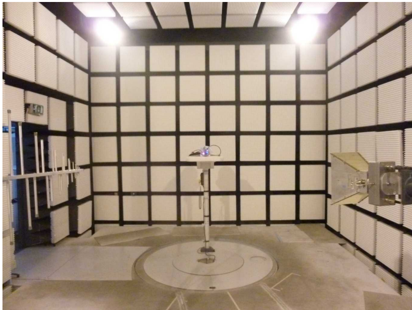
Photo 5: EUT at the anechoic chamber
