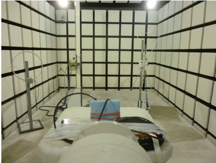
Photo 3: EUT at the anechoic chamber
