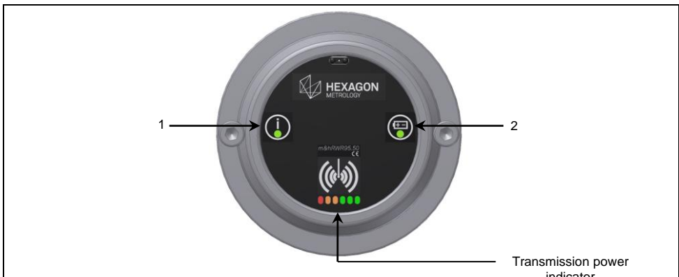
Fig. 20 LED Indicators of RWR95.50
