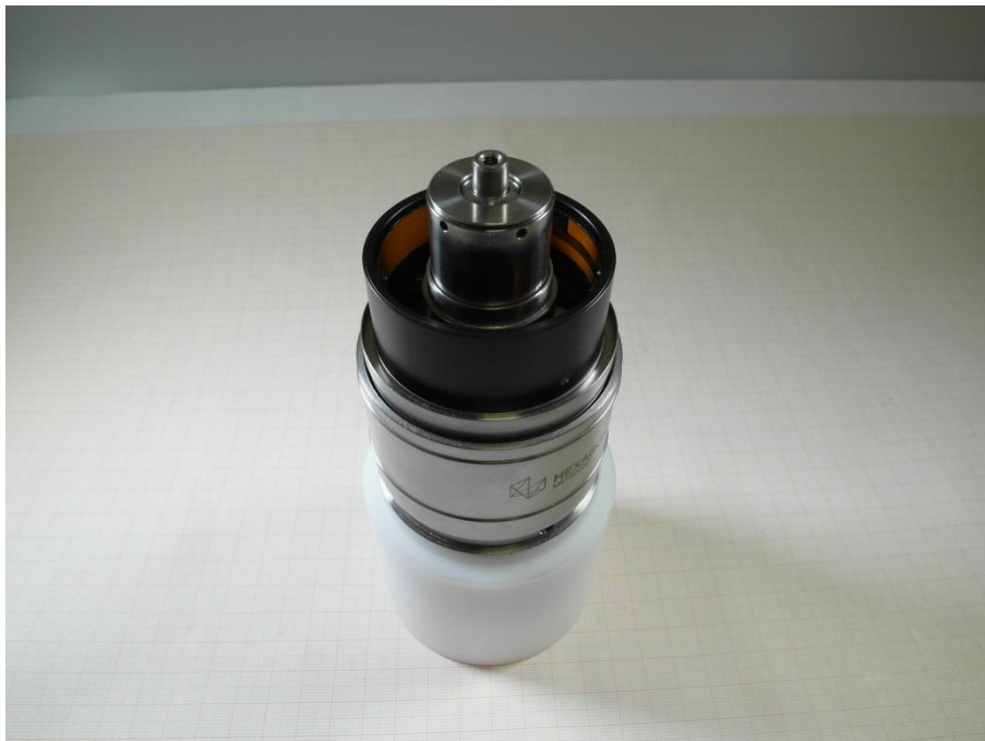
Photo 5: antenna holder without shelter
