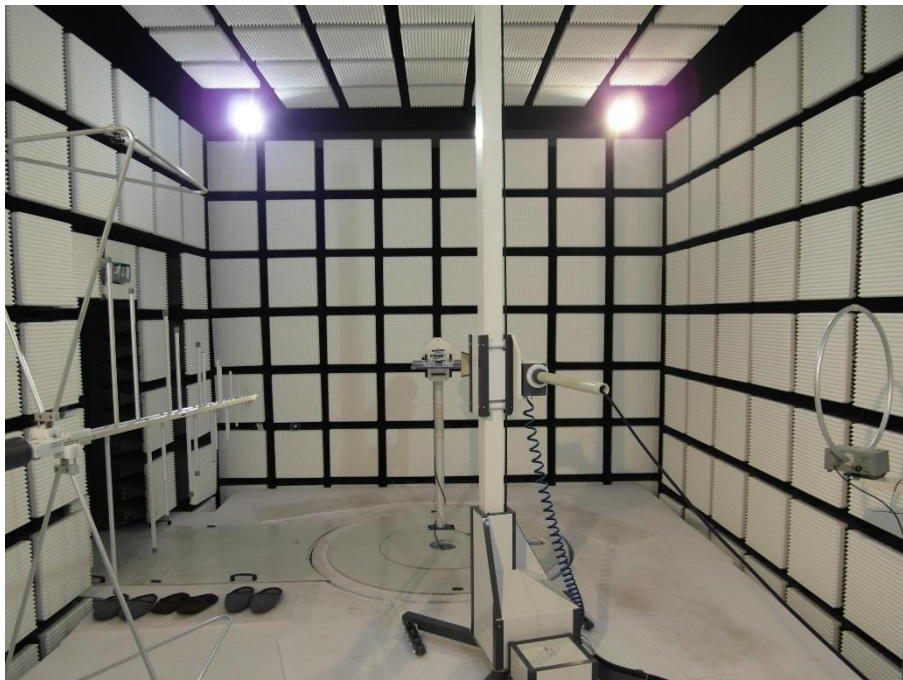
Photo 5: anechoic chamber overview
