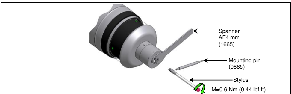
Fig. 8 Stylus change with measuring unit MY21.00
