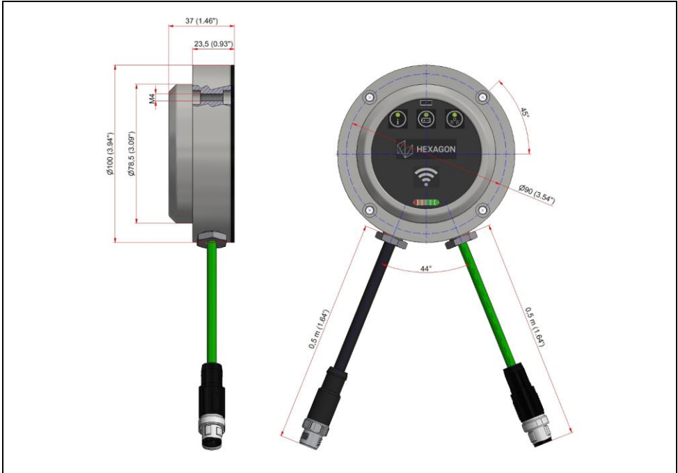
Fig. 2 Dimensions RC-R-100-R (cable outlet radial)
