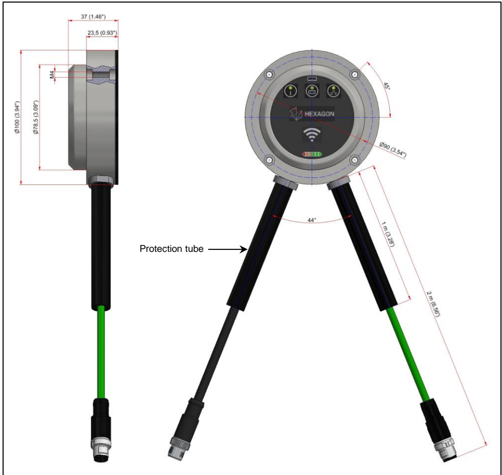
Fig. 3 Dimensions RC-R-100-R-PT (cable outlet radial)
