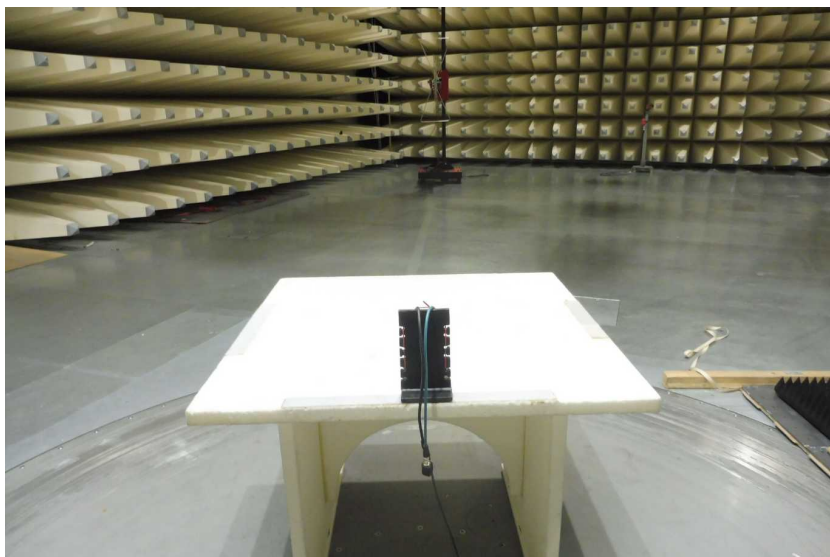
EUT at the semi-anechoic chamber
