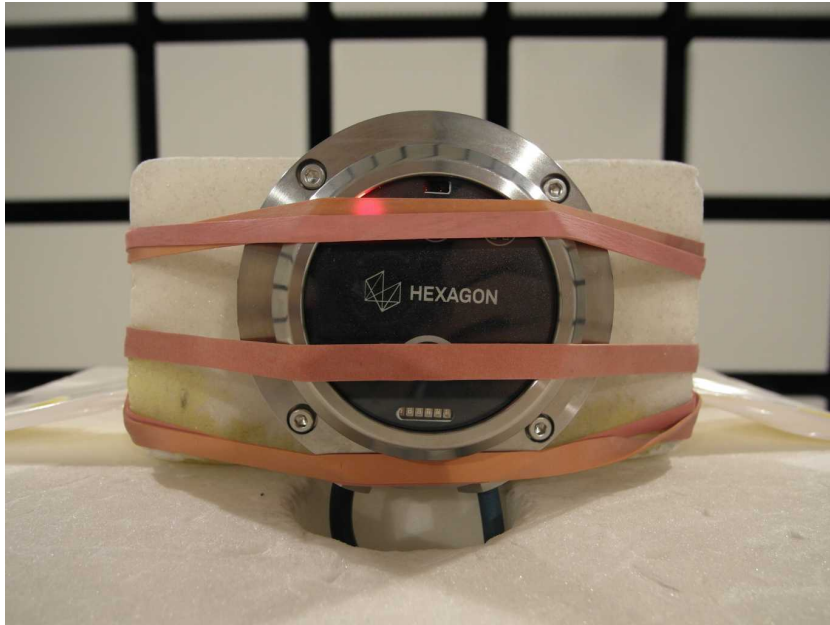
EUT at the anechoic chamber
