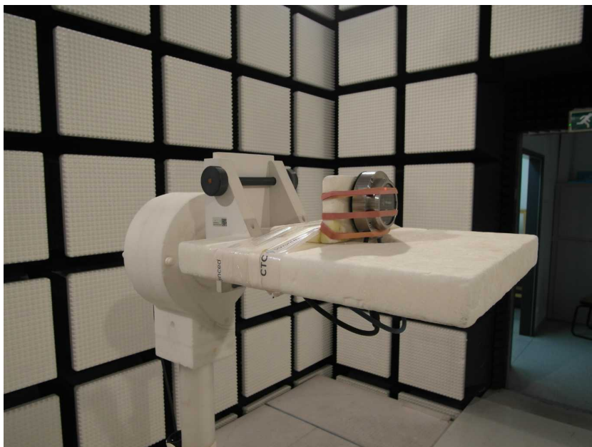
EUT at the anechoic chamber
