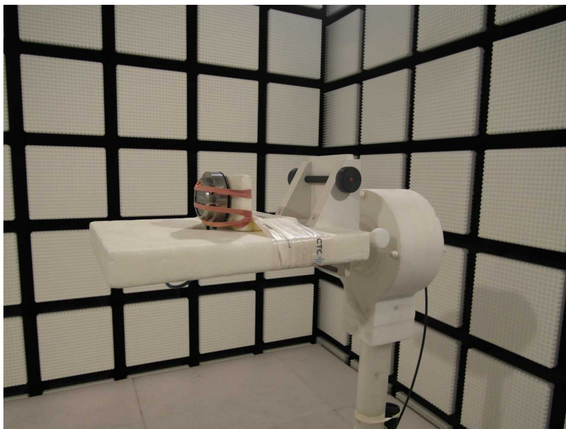
EUT at the anechoic chamber
