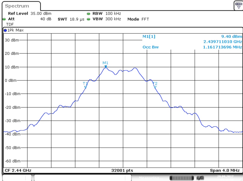
Figure 57: 99% OBW, Channel 19 mid, power setting 145, PHY 125k coded
