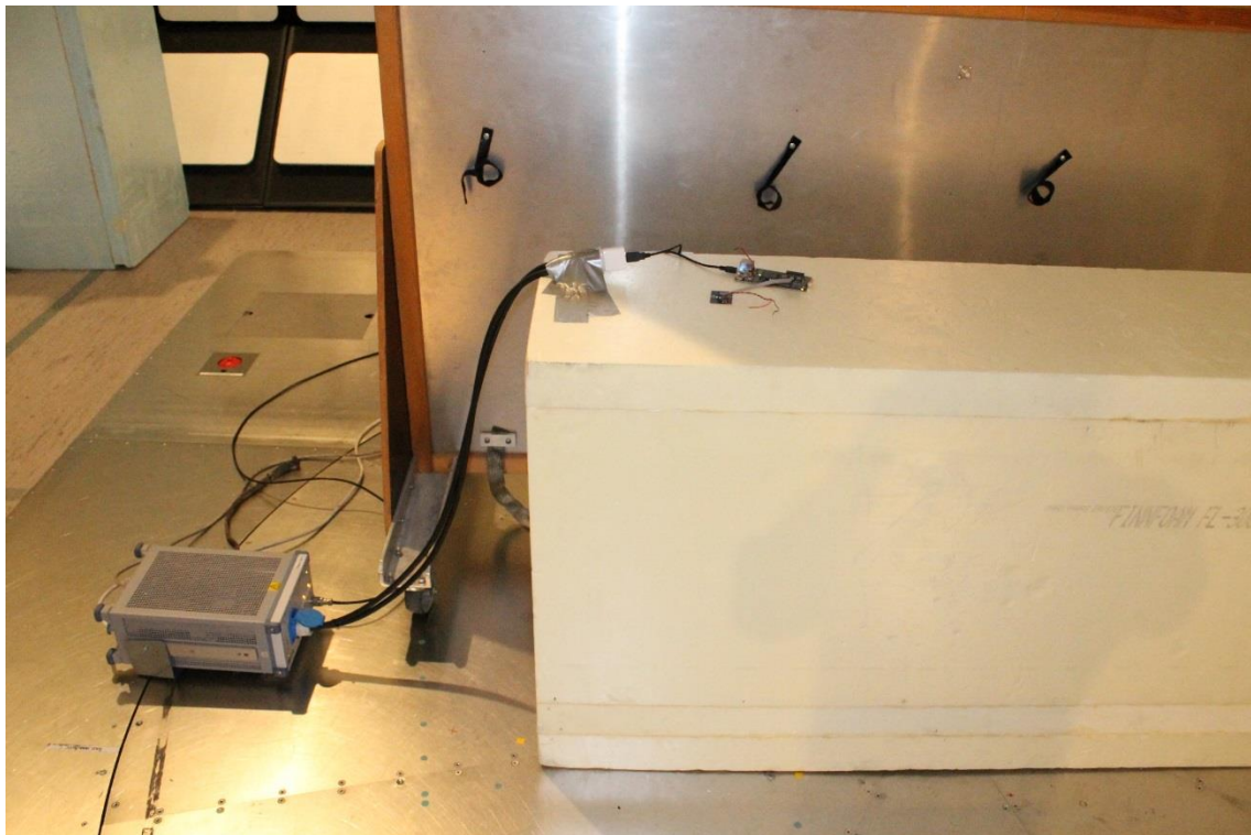
Photograph 10. Conducted Emissions for DUT 2, BGM13SA
