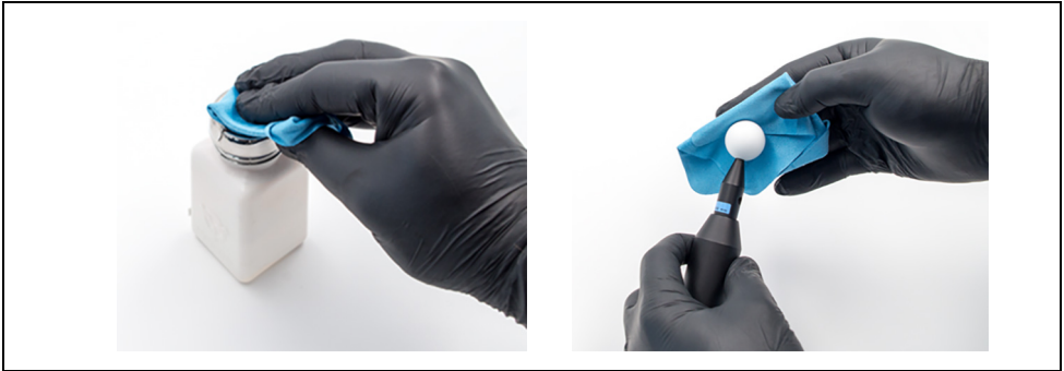
Fig. 19 Wet cleaning the calibration sphere with isopropyl alcohol
