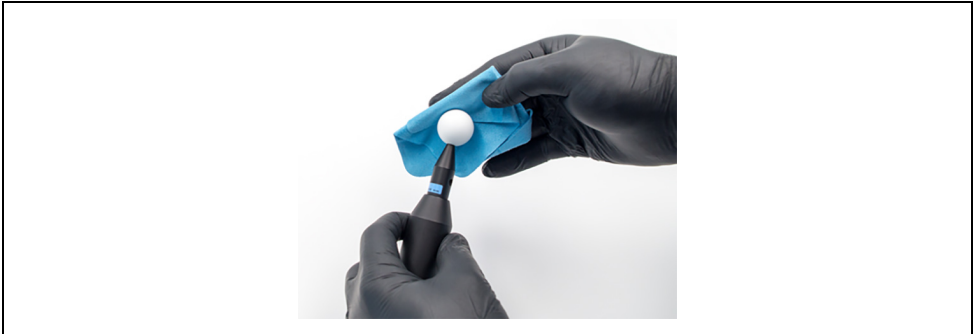
Fig. 18 Dry cleaning the calibration sphere with a micro-fibre cloth
