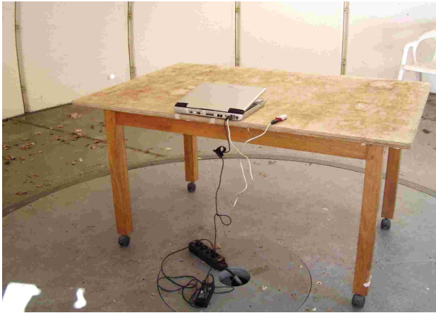
Detail view (EUT used with the USB extension cord)
