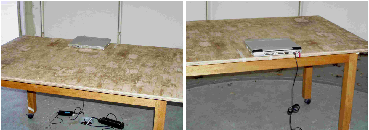
EUT 80cm above the ground reference plane without USB extension cable
