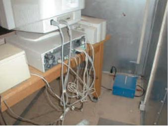
The EST and auxiliaries are set on the no-conductive table of 80 cm height.
